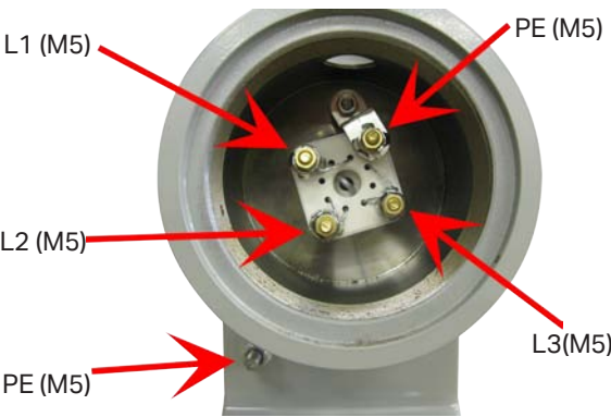
Fig. 6 ERB 3-phase electrical connections
